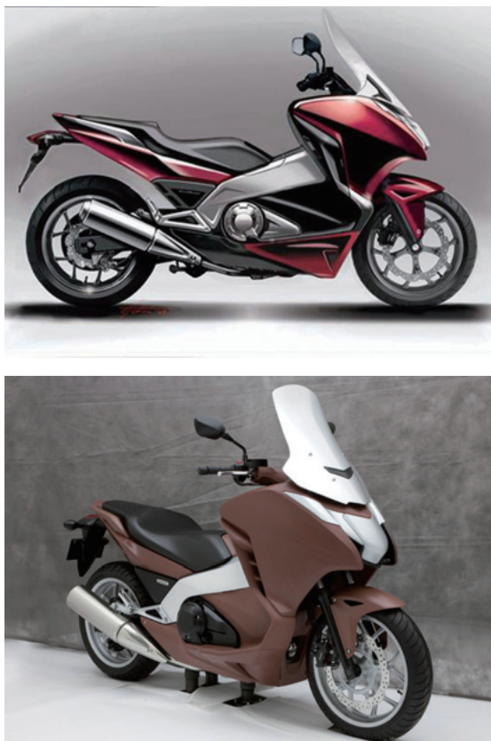
Fig. 3 Concept sketch and clay model of INTEGRA
