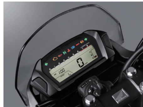
Fig. 14 Meter display unit of NC700S
