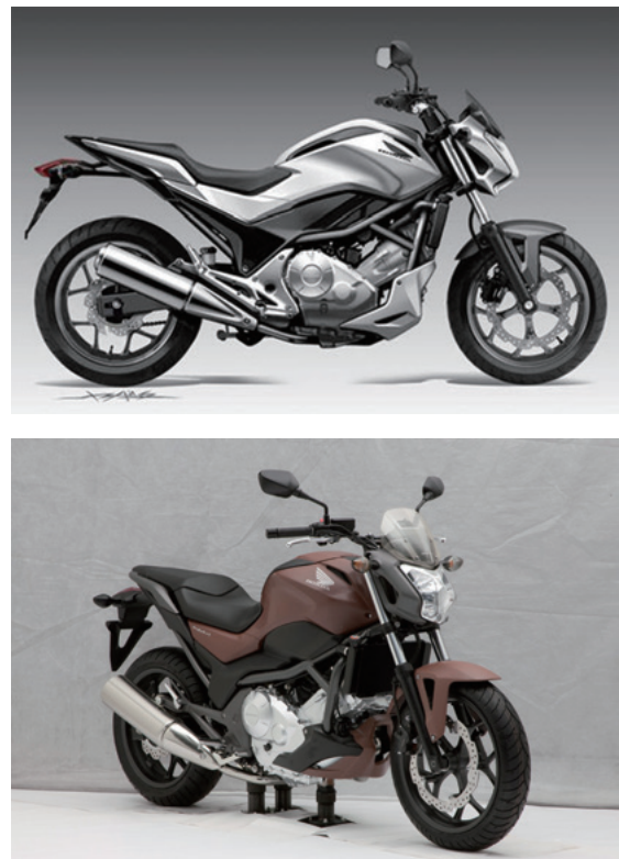
Fig. 1 Concept sketch and clay model of NC700S
