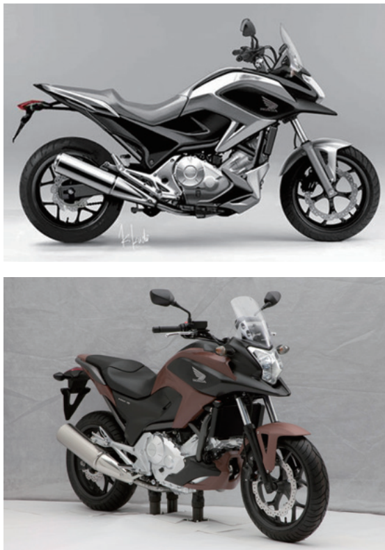
Fig. 2 Concept sketch and clay model of NC700X
