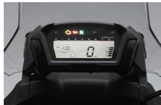
Fig. 15 Meter display unit of NC700X
