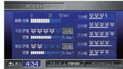
Fig. 11 Vehicle onboard display for eco-driving rating results
