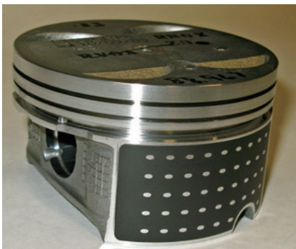
Fig. 7 "Moly-Dot" piston skirt coating
