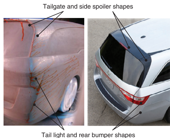
Fig. 13 Wind tunnel development of rear flow separation
