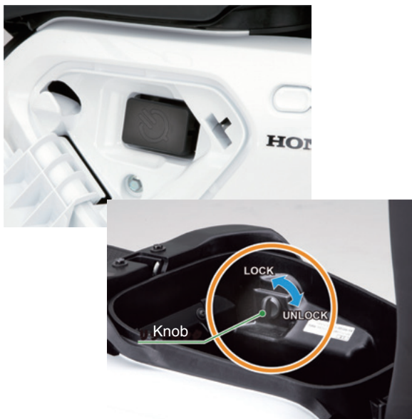
Fig. 7 Charging connector and lock of charging receptacle lid
