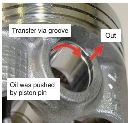
Fig. 9 Oil transfer path in piston pin hole
