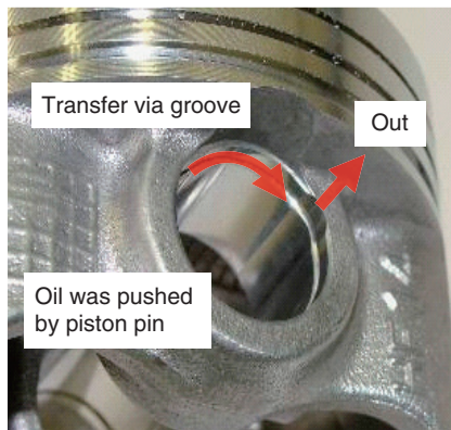
Fig. 9 Oil transfer path in piston pin hole
