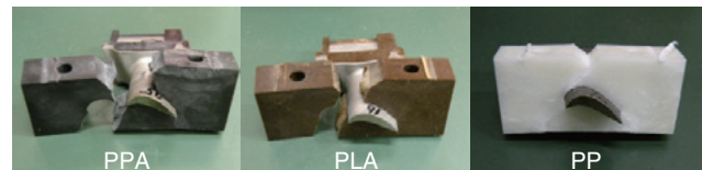
Fig. 8 Results of breaking method with notch
