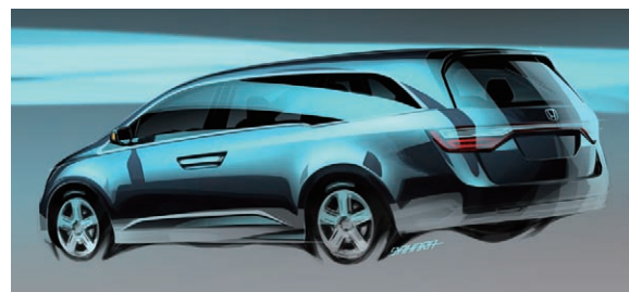
Fig. 7 Styling sketch of rear shows car-like wide tail lamp design
