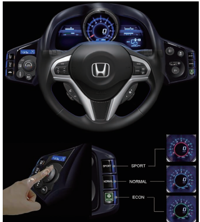
Fig. 18 Meter cluster panel
