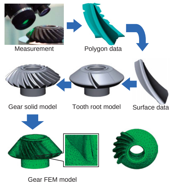
Fig. 5 3D model making process
