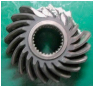
Fig. 16 Status of gear damaged in durability test
