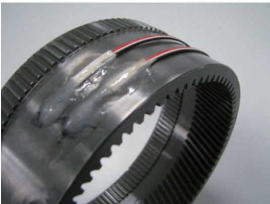
Fig. 5 Position of strain gauge
