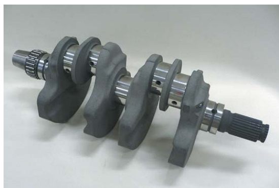
Fig. 21 Crankshaft with new geometry for new V-4 cylinder engine
