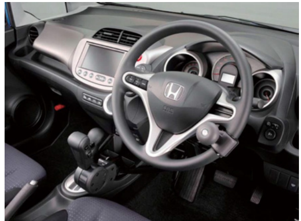
Fig. 5 Auxiliary driving device operated by hand (New type)
