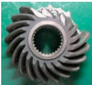
Fig. 16 Status of gear damaged in durability test
