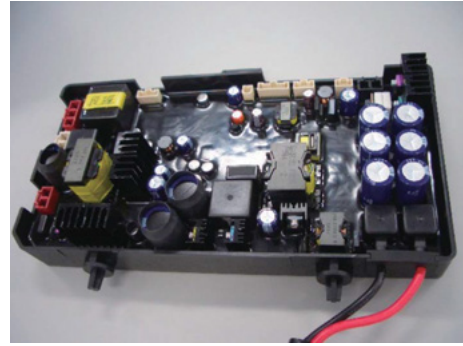
Fig. 11 DC-DC converter unit
