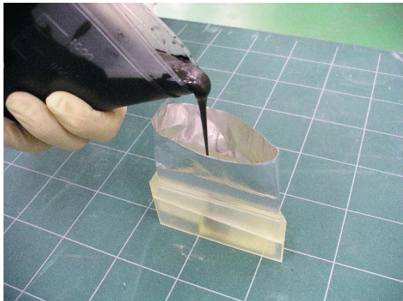
Fig. 14 Casting of core
