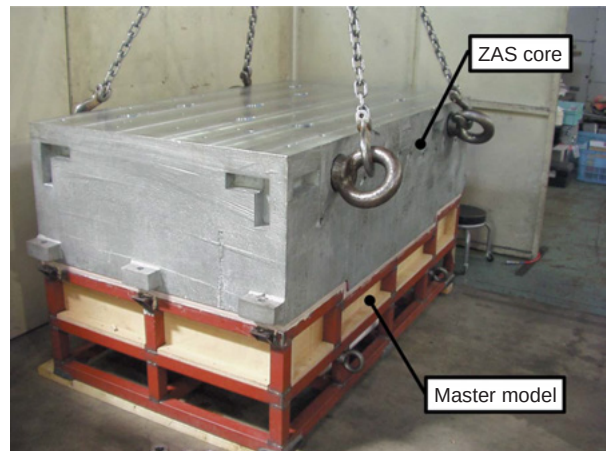
Fig. 12 Combination of master model and ZAS core
