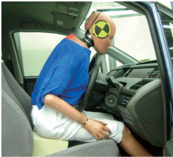
Fig. 10 AF 5 % dummy set for measuring impact force of air bag
