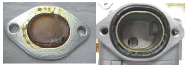
Fig. 15 Residue that drained into cup (use for 50 hours)
