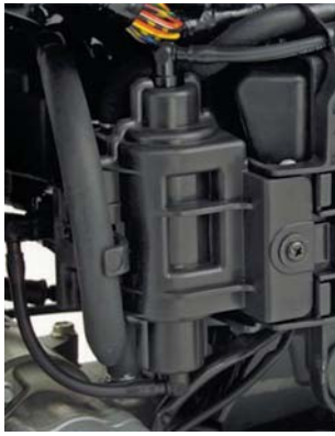
Fig. 23 External view of stream of replacement filter
