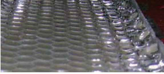
Fig. 8 Honeycomb layer torn away with cladding (note undisturbed layer of adhesive present under torn honeycomb layer)
