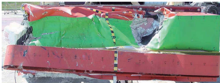
Fig. 1 Typical damage to honeycomb barrier seen after FMVSS 301 high speed rear crash test
