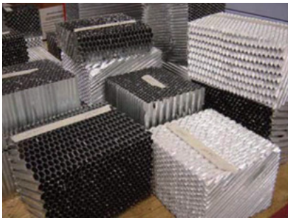
Fig. 4 Samples cut from honeycomb block at different angles
