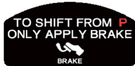
Fig. 11 Shift lock in operation
