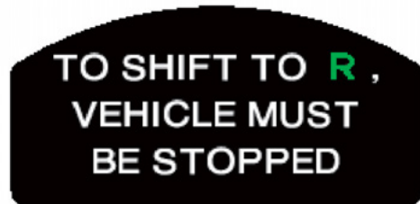
Fig. 12 R inhibitor in operation
