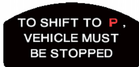
Fig. 13 P inhibitor in operation
