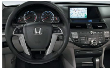
Fig. 8 Accord sedan instrument panel
