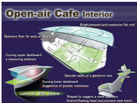
Fig. 12 Approach to interior design
