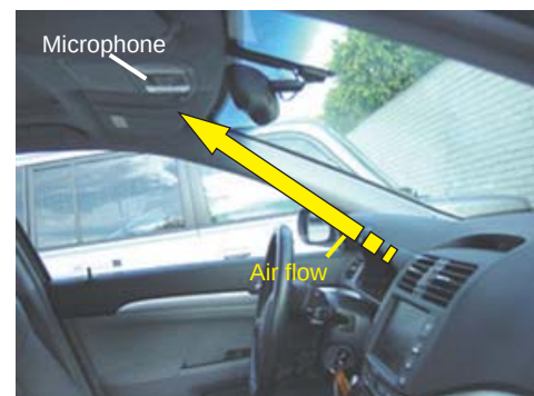
Fig. 5 Direct airflow from air conditioner
