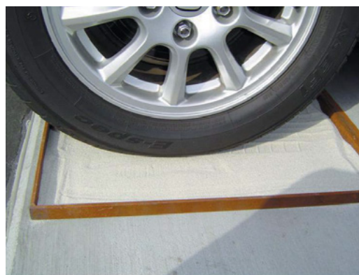
Fig. 7 Measuring resistance through tires with sand between tire and concrete pad
