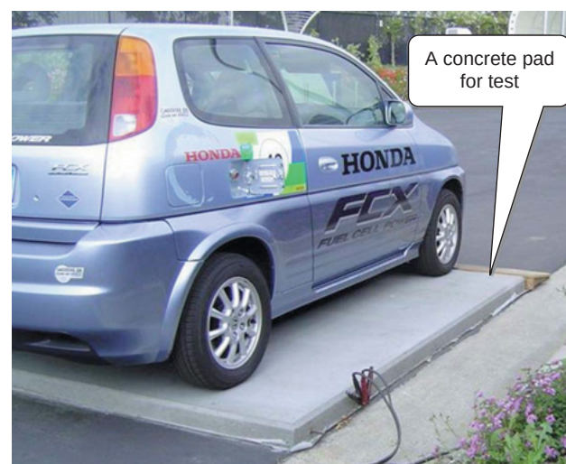
Fig. 5 Measuring resistance through tires parked on concrete test pad
