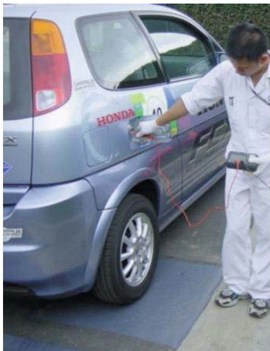
Fig. 6 Measuring resistance through tires parked on conductive painted test strip
