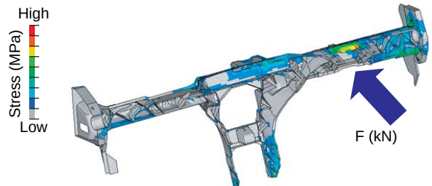
Fig. 3 Frontal offset static load CAE result (Stress distribution)
