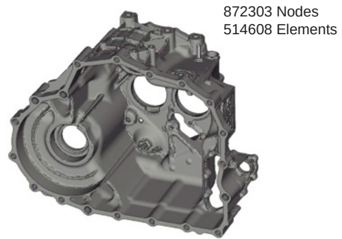
Fig. 9 FE model based on CAD
