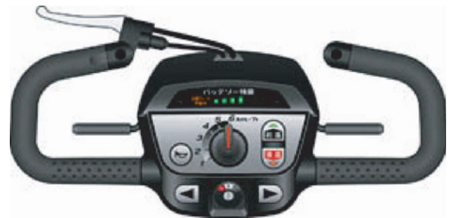
Fig. 8 Design sketch of control panel
