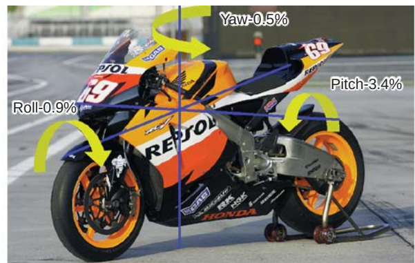
Fig. 12 Result of moment of inertia
