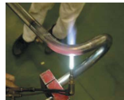
Fig. 10 Manual bending by specialist
