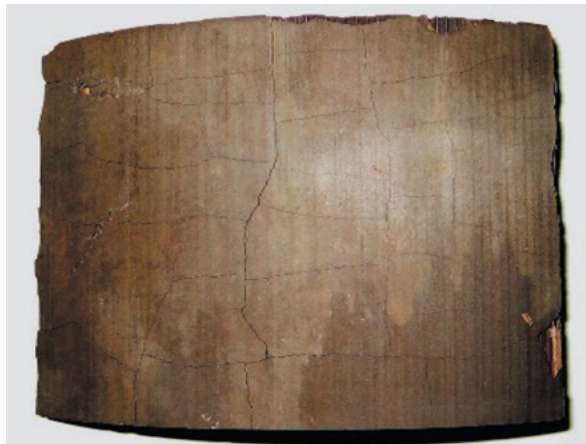
Fig. 3 Surface crack after 830°C x 300Hr aging
