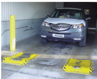
Fig. 13 Sweeping frequency bump in vehicle build plant
