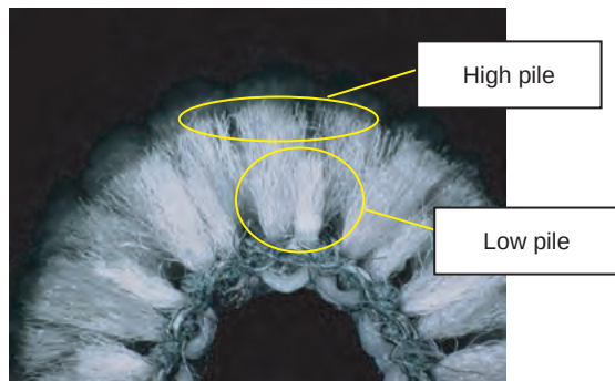
Fig. 10 Typical construction of dual-layer pile
