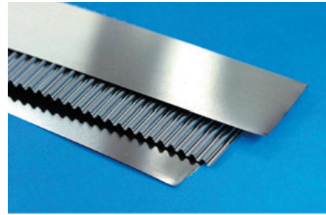
Fig. 3 Flat foil and corrugated foil
