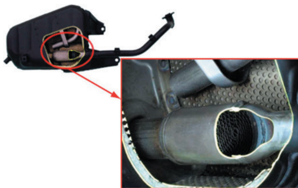
Fig. 2 Outline view of muffler with metal-honeycomb catalyst on small sized two-wheeled vehicle for India model
