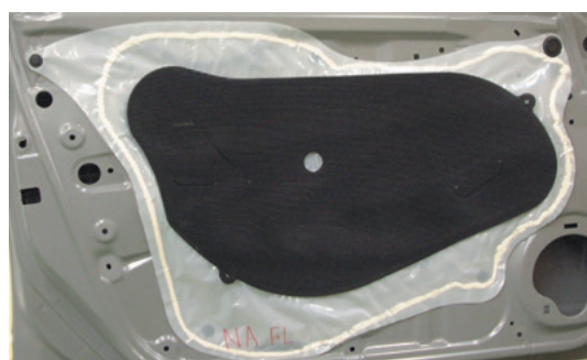
Fig. 9 Heat cycle test result (door panel)
