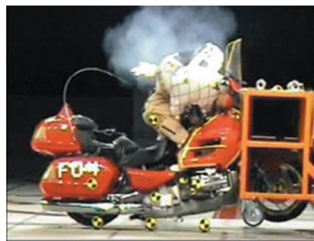
Fig. 20 Under-ride impact test
