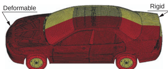
Fig. 4 Opposing vehicle model for front-side impact case
