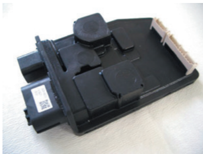
Fig. 8 Outside view of a hot melt molded ECU
