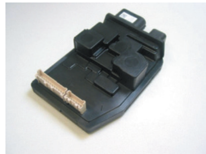
Fig. 21 View of ECU
