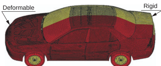
Fig. 4 Opposing vehicle model for front-side impact case
