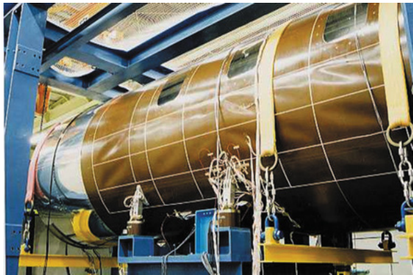
Fig. 16 Skin buckling at limit load
