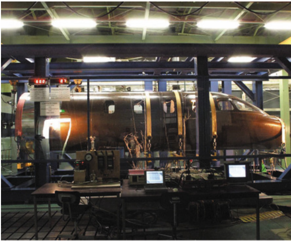
Fig. 15 Cabin component test
