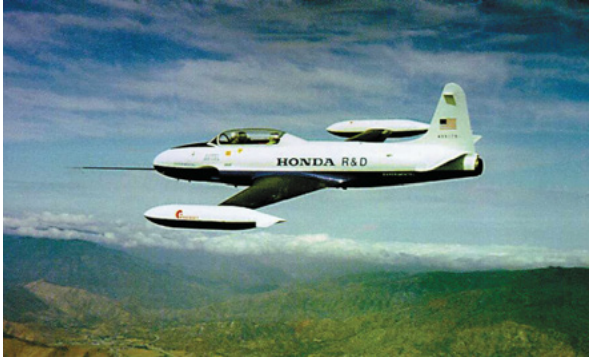
Fig. 4 T-33 aircraft modified for NLF flight test
