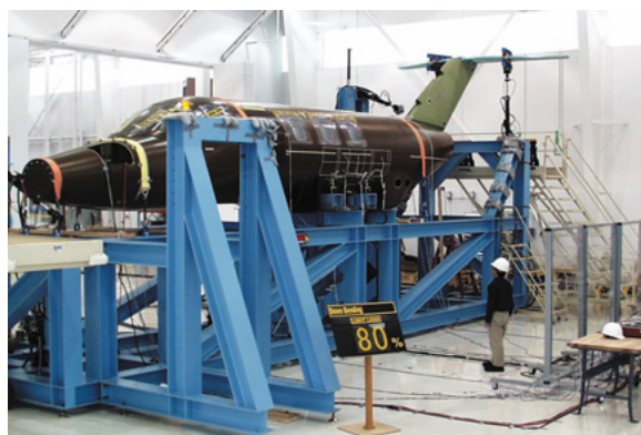
Fig. 17 Fuselage proof test
