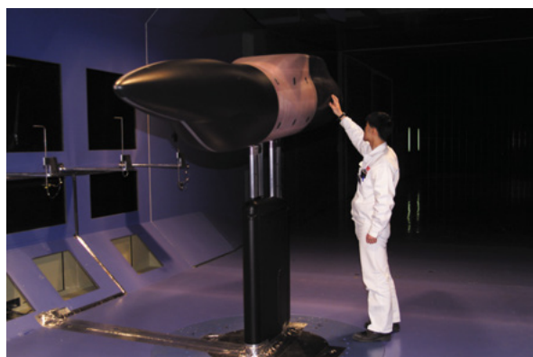
Fig. 9 1/3-scale fuselage model for NLF nose test
