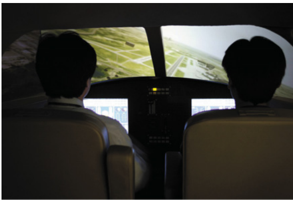
Fig. 12 Honda flight simulator(HNAFS)
