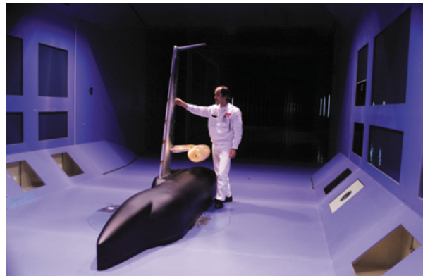
Fig. 6 1/3-scale low-speed wind tunnel model
