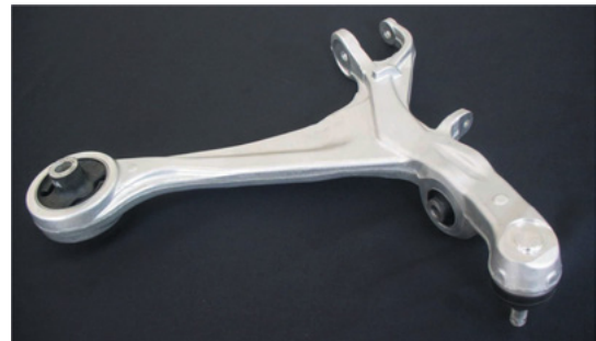
Fig. 16 Front lower arm
