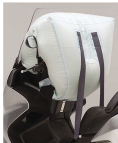
Fig. 6 Prototype airbag system for large scooter
