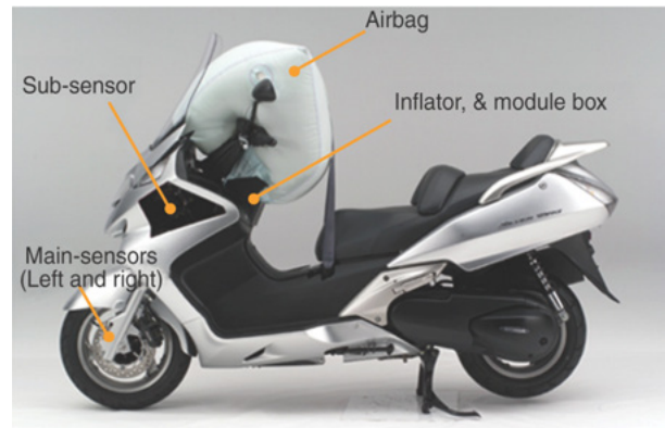
Fig. 5 Large scooter with prototype airbag system
