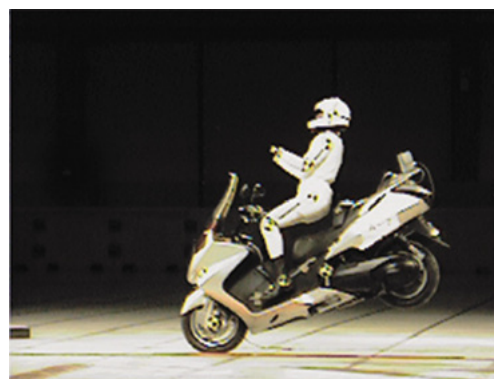
Fig. 2 Motorcycle and dummy in simulated curb ride over test
