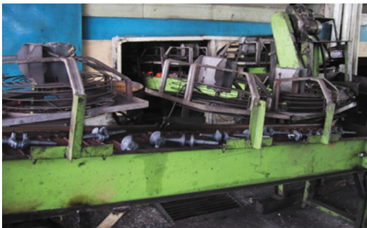
Fig. 2 Fan cooling after hot forging
