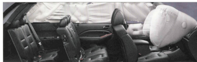
Fig. 5 Deployed front airbags, side airbag and side curtain airbag
