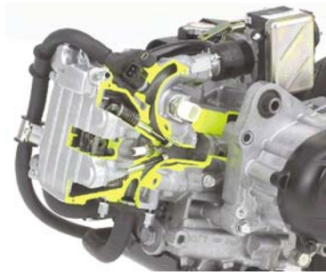
Fig. 21 Cutaway model of 50cm 3 four stroke engine with PGM-FI system
