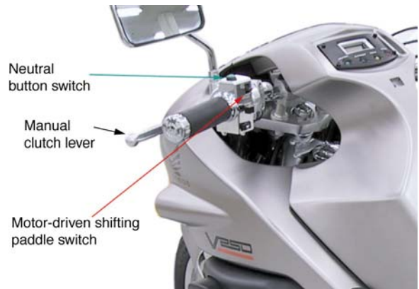
Fig. 13 Manual control gearshift system
