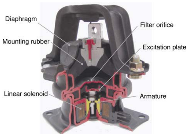
Fig. 12 Cutaway view of ACM
