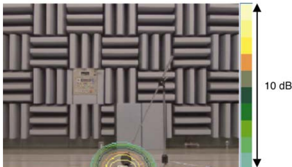
Fig. 6 Result of single source test (loudspeaker, 1 kHz)
