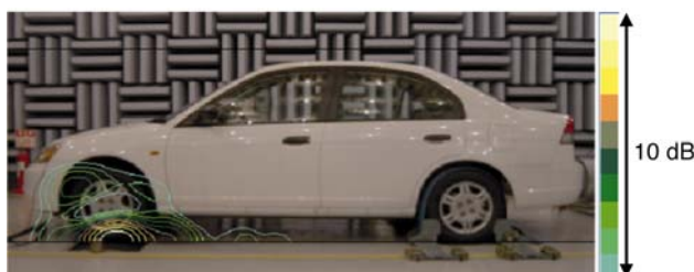
Fig. 17 Result of beamforming (without exhaust noise radiation)
