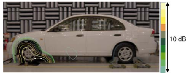
Fig. 12 Result of beamforming analysis
