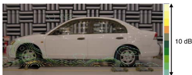
Fig. 16 Result of beamforming analysis (with exhaust noise radiation)
