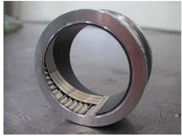
Fig. 12 Air foil bearing (Cut model)
