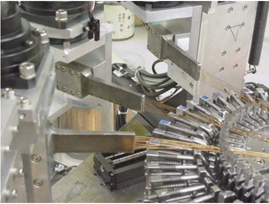
Fig. 5 Nozzles for winding of three phases
