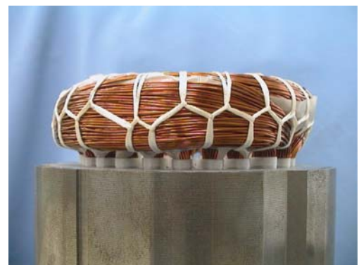
Fig. 3 Winding overhang produced by insert coil Machine
