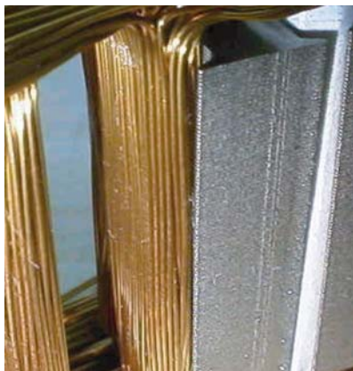
Fig. 11 Winding aligned inside a slot
